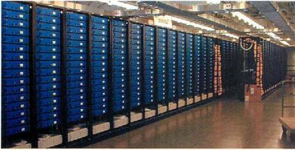
Square Pictures' 1,160-CPU rendering farm was custom built for the movie. It includes 960 933MHz Pentium III systems with 768MB of RAM each, plus 150 Silicon Graphics Origin 200 systems with 4GB of RAM each.
